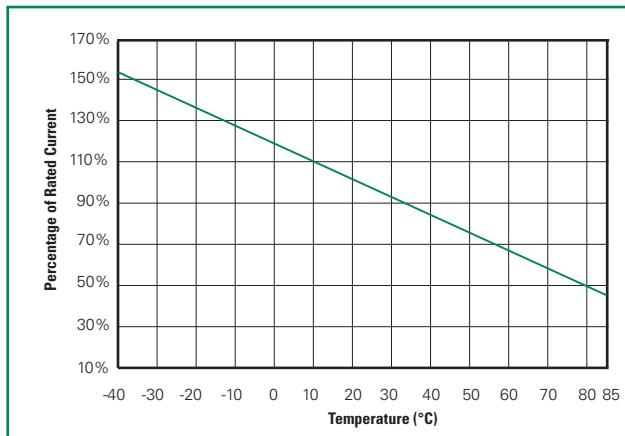
The average time current curves and Temperature Rerating curve performance is affected by a number of variables, and these curves provided as guidance only. Customer must verify the performance in their application.
